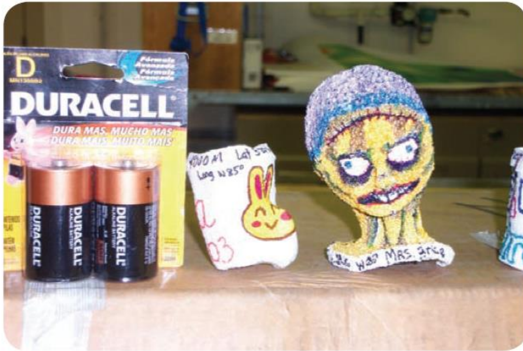
Figure 2-5 PRESSURE. To demonstrate the pressure in the sea's depths, this wig head, originally the size of a human head, was lowered to a depth of 4,000 meters (13,200 feet). The pressure at this depth is so great that it compressed the Styrofoam to the size you see in this photograph.
